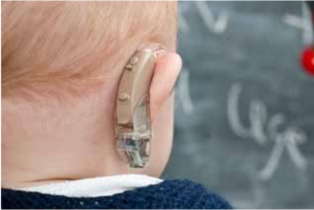
Picture 3: Picture of an infant wearing a regular-sized hearing aid with an FM shoe attached.
